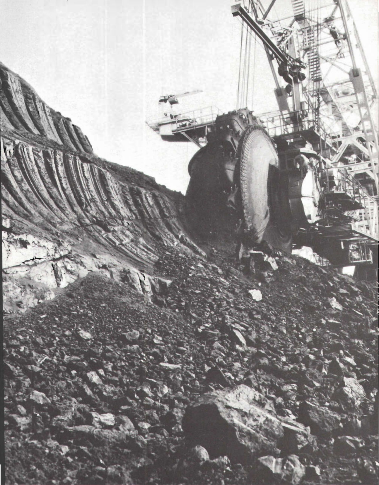
A bucket-wheel coal dredger in operation at the Morwell open cut in the La Trobe Valley.
